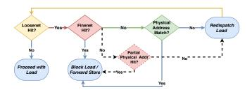
Figure 3: The dependency check logic: *loosenet* initially checks the least 12 significant bits (page offset) and the *finenet* checks the upper address bits, related to the page number. The final dependency using the physical address matching might still fail due to partial physical address checks.
