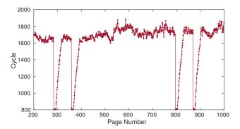
Figure 14: The effect of SPOILER on TLB flush. The execution cycle always increases for 4 kB aliased addresses, except for some of the virtual pages inside in the store buffer where we observe step-wise hills.
